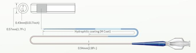
\*Hydrophilic coating (M coat) is not applied to the proximal portion of  $60\ cm$ .
